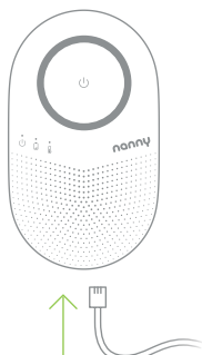
Fig. 9 Connecting the connection cable to the control unit
